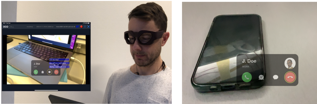
Figure 3: Controlling an incoming call by performing various head and facial movements.
