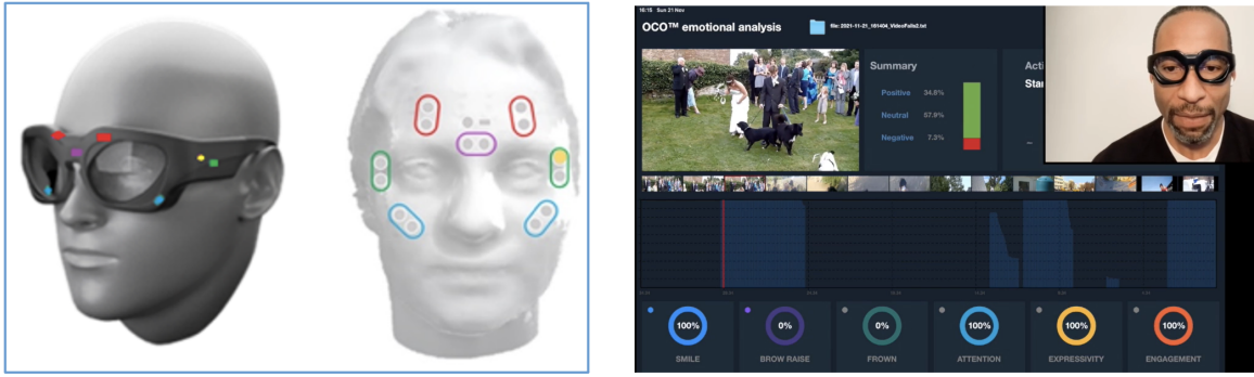
Figure 1: . OCOsense™ glasses and sensor placement (left), the mobile application (right). The coloured rectangles represent the OCO™ sensors within the frame, upon major facial muscles: frontalis (red), zygomaticus (blue) and corrugator (purple). The green OCO™ sensors are positioned over the temples. Also, there is a 9-axis IMU and altimeter - yellow circle. The stimuli emotional analysis screen on the mobile device is shown with the expression/gesture detected from the wearer (right).
